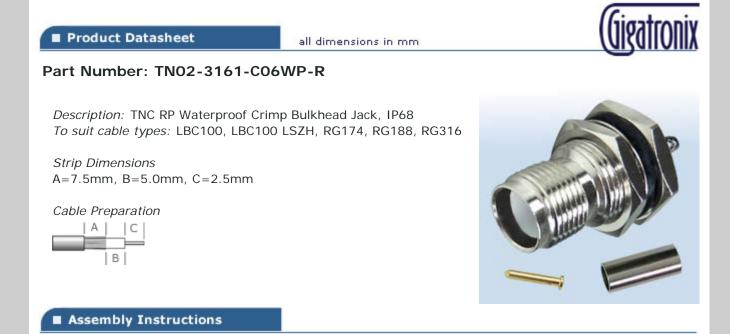
1) Slide the ferrule onto the cable and strip the cable to the dimensions as shown, taking care not to nick the centre conductor or braid.
